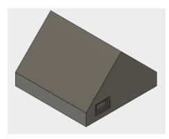
7. Door: Create a box on the other side for where a door would be (length and width don't matter as long as it connects to the base) and type in -3 for the height.
