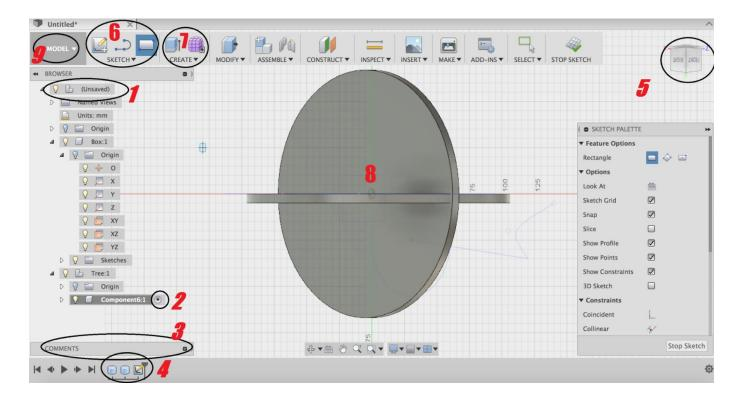
1. By right clicking on a component, you will find a list of options that allows you to create new components, remove old ones, or manage current settings.
