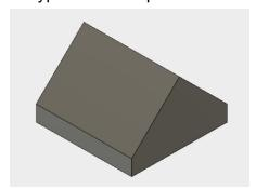
5. Window: Go to "create" -> "box", and draw a rectangle on the left front face (any width and length is fine). For the height, type in -2 and press enter.
