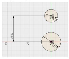
10. Press the "O" key (offset - found under "sketch"). Click on the edge of the circle, and type in 3, then press enter. Do this for both objects.
