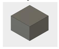
3. Select "modify" -> "chamfer", and then click on the left and right edges on the top of the box.
